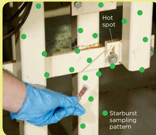
Figure 5. Vector Sponge/Swab Sampling Starburst Pattern Around the Initial Salmonella Presumptive Positive Site.
